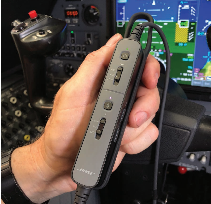
The ProFlight headset incorporates three acoustic profiles: Low, Med, High. Each are tuned to a particular combination of frequency attenuations or cancelling.
