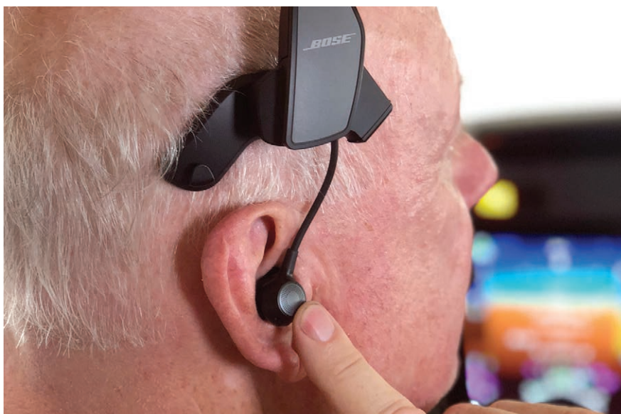
Bose incorporated instant ANR reduction by way of double tapping either ear piece.
